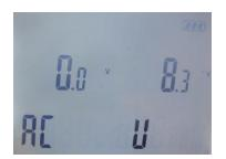
The moment shown AC (or DC) appears on the left bottom of the screen, indicating the voltage of the measured mains is AC (or DC). The left-hand side of the screen shows the mains voltage value, while the right-hand side shows the voltage value of internal battery.
