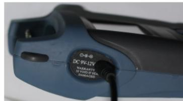
appear in LCD. when the battery is going to run out, the power volume indicator will blink once a second, the device will automatically power off after the indicator blinks for ten times; if so, you can insert the device into supplied charger for charging (see the Figure on the right).
